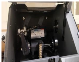
Fig.2 (a): SPEX shaker mill each
